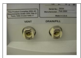
In the back of the Laser there are two white fittings labeled "VENT" and "DRAIN/FILL". They are underneath the serial number and to the left of the power cable. With your laser you received a "Fill Funnel Kit" that consists of two hoses with white fittings on one end. One is blue and it has a yellow funnel at the other end, and the other one is black.
