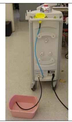
Connect the Blue hose first. Keep it high to prevent draining water out. The best way to do that is to thread the hose between the handle and the console, to support the funnel at the proper level. Plug the other end of the hose to the right fitting labeled "DRAIN/FILL" (see pictures). Fill funnel with distilled water. Always keep water in the funnel to prevent air bubbles from entering the hose.
